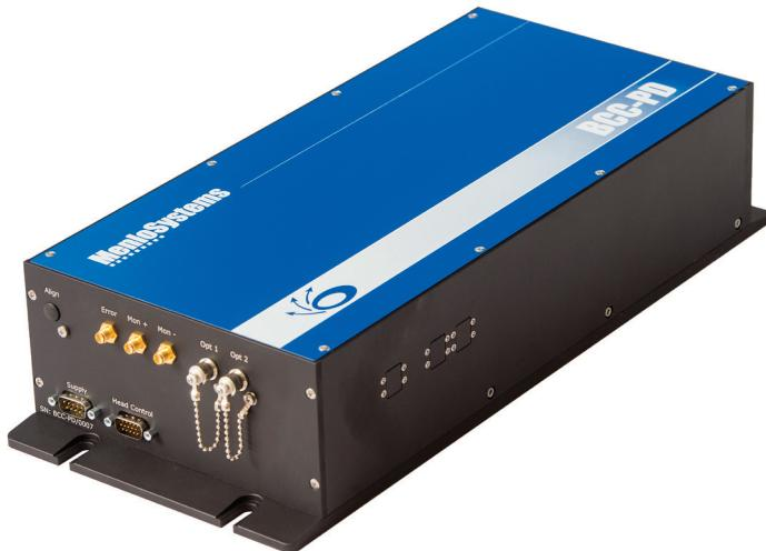
The high resolution optical balanced cross correlator is optimized for detecting the timing error between the reference pulse train and a laser client system with ultra-high sensitivity. The balanced detection makes the system more robust reducing the phase deviation from unintentional amplitude variations (AM-PM conversion). The BCC-PD is required for high level synchronization of femtosecond laser systems to a reference pulse train.
