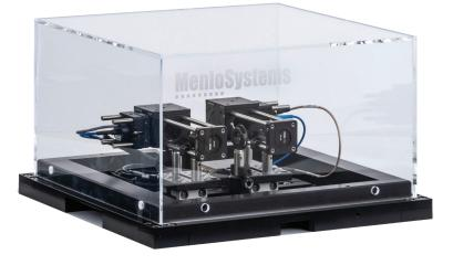
Menlo Systems provides a complete purge box add-on compatible to all terahertz spectrometers and the state-of-the-art Menlo THz optics. It provides a ready-to-use enclosure made of transparent Plexiglass nicely mounted to a solid metallic base. The enclosure offers cable feedthroughs, handles for lifting, and 2 connectors for standard 6 mm purging tubes.
