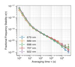
We believe in fully phase-locked systems, being the only path for phase-coherently transfer the purity from one specific optical frequency to all frequencies. Here the robustness of our phase-lock-loops is measured, demonstrating the negligible additive noise and the full control of the disciplined CW lasers.
