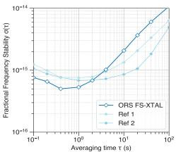
The rack-mounted ORS of the FC1500-Quantum is characterized in terms of single-sideband optical phase noise power spectral density and fractional frequency stability. Menlo Systems carries on detailed analysis for each system to guarantee ultimate performance and uninterrupted operation. A three-cornered hat technique is used to provide absolute noise analysis of the ORS.
