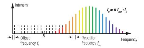
The optical comb frequencies  $f_n$  are defined by the repetition rate frequency  $f_{rep} = 250$  MHz, the carrier envelope offset (CEO) frequency  $f_0$  and an integer number n.
