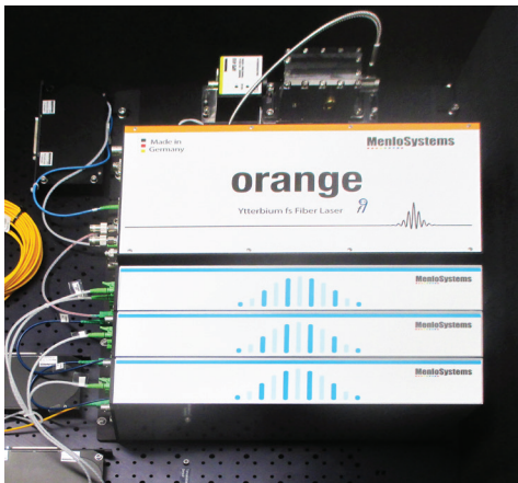
Oscillator with CEO stabilization above and filtering cavities below (left), AstroComb system control rack (center), and the spectral flattening unit (right)
