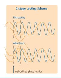
The phase relation is defined through the fundamental lock. Locking is done at higher harmonics for superior phase sensitivity.
