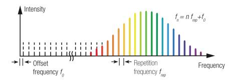
The optical comb frequencies  $f_n$  are defined by the repetition frequency  $f_{rep}=100$  MHz, the offset frequency  $f_0=10$  MHz and an integer number n.
