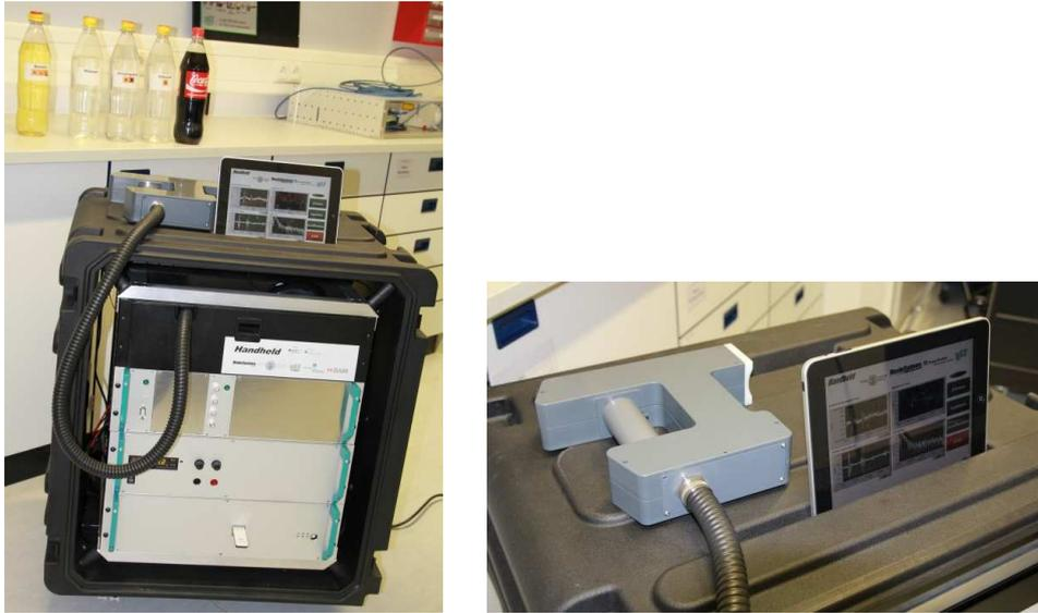
**Figure 2:** Handheld portable THz spectrometer for the detection of hazardous fluids (left picture) with measurement head (right picture)
